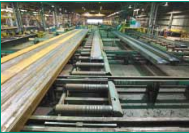
Only Peddinghaus provides material handling flexibility to easily transfer sections to work stations located to the left, right, or down the center.
