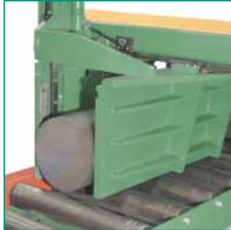
The rigid clamp enables round stock or pipe to be clamped securely for accurate cutting.
