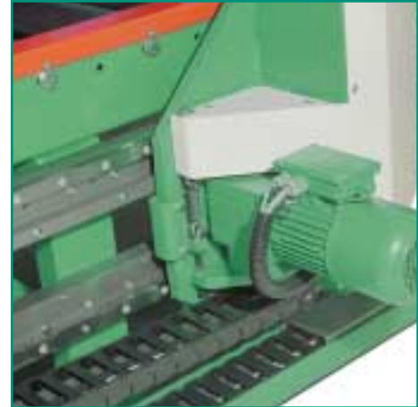
The powerful infeed drive motor insures efficient feeding of heavy or oversized material.
