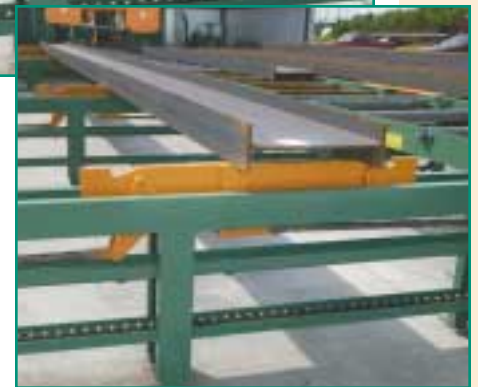
The unique quiet glide carriage assembly selects the section needed.
