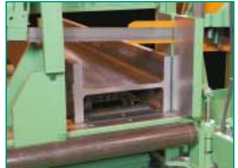
Material is rigidly clamped...yet easily transported with a unique lifting and lowering bed mechanism.
