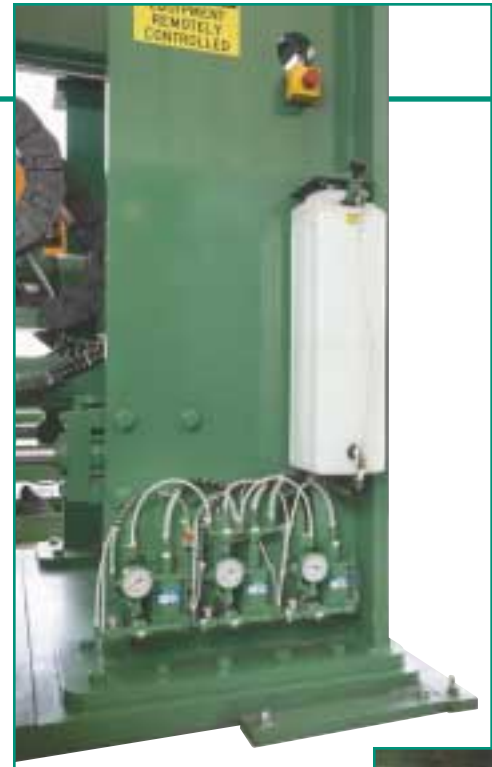
Peddinghaus provides spindle induced air mist drill cooling which eliminates expensive flood coolant clean up. This process saves tooling costs, and expedites welding and painting operations.
