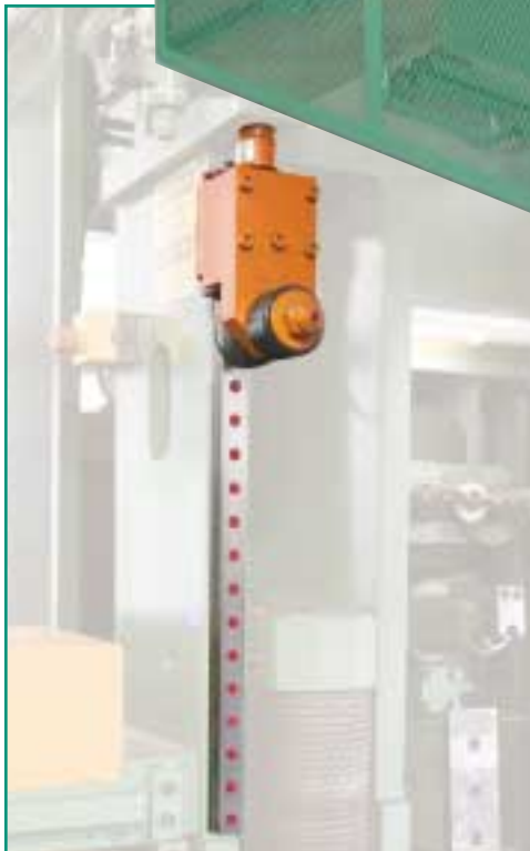
Precision rails reduce maintenance costs by housing positional feedback devices that insure accurate hole locations.
