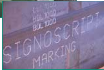
The integrated Signo Script Marking system employs a carbide mill cutter, which provides legible part identification regardless of depth, height, or part number orientation.
