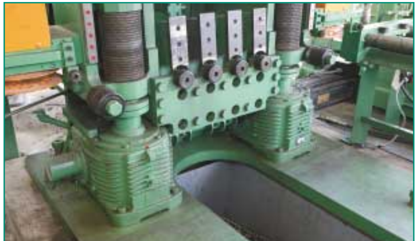
The robust gearbox design of the BDL drills provide crisp positioning accuracy for the heaviest rolled or fabricated sections to the lightest structural members.
