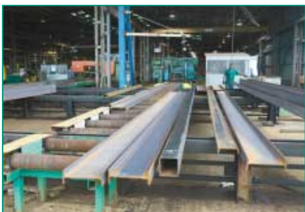
Various sections sizes and shapes are stored and easily selected to maximize productivity per job.
