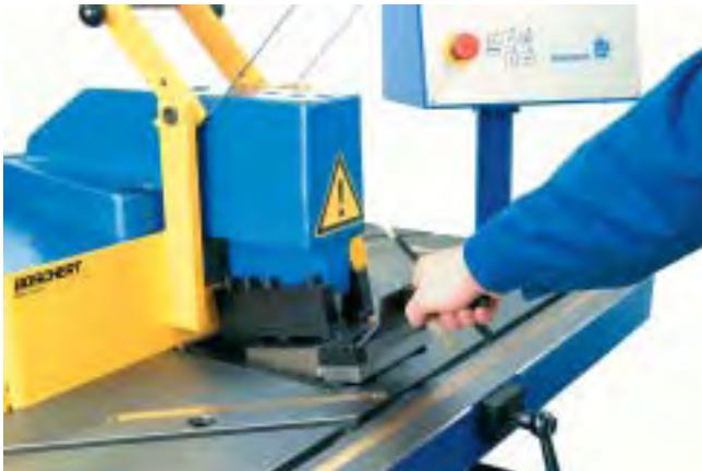
Silver Eagle QUICK with quick-change tool sets for special cuts and notches
